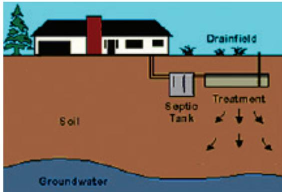
Septic tanks and cesspools treat household wastewater only minimally, removals of pollutants such as nitrogen are less than 20% than that of a wastewater treatment facility.
