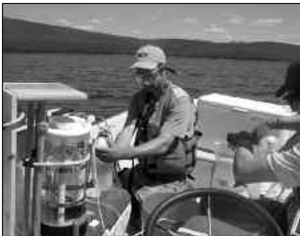
Figure 7: Limnology is the science of freshwater lakes and reservoirs and limnology sampling is typically done at several depths to characterize the different chemical, physical and biological characteristics of the layers that develop with seasonal warming, a condition referred to as stratification. DEP samplers are shown on Ashokan Reservoir.
