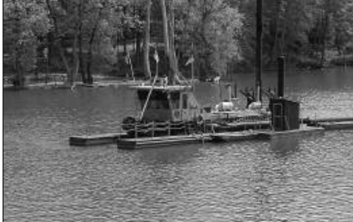
A Canal Corporation hydraulic dredge operating on the Champlain Canal section
