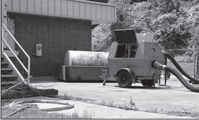
A portable pump runs to bypass sewage at the Deposit, NY plant.
